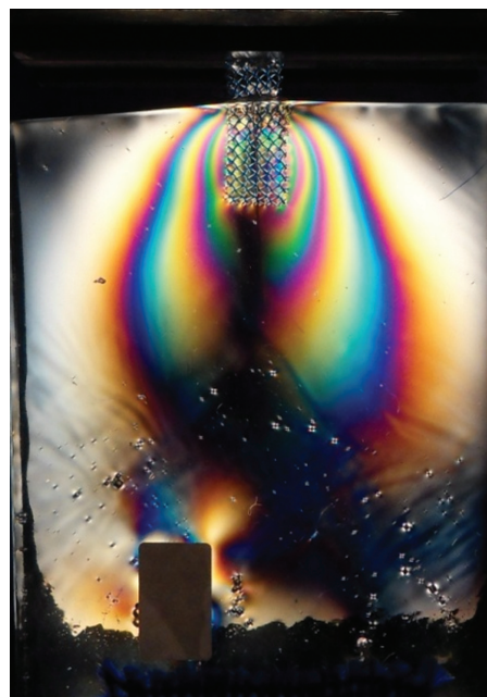
Figure 5 Isochromatic lines in a tension test of the GC mesh embedded in gelatin.
