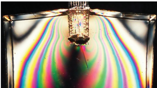
Figure 12 Rupture of the gelatin at the end of the SD mesh.
