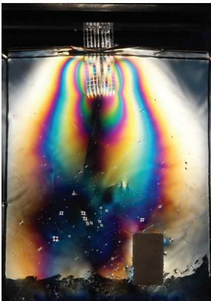
Figure 3 Isochromatic lines in a tension test of the SD mesh embedded in gelatin.
